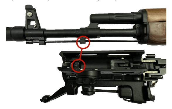
Step 2: Push up the grenade launcher to the AK outer barrel.
