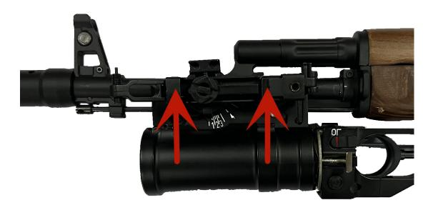
Step 3: Slide the grenade launcher backwards
