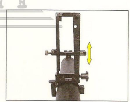
Push the button on the left side of the rear sight to unfold the folding ladder-style leaf-type sight. User can adjust the shooting range indicator by loosening the screw button. (Shooting range scale on indicator is not accurate for the Airsoft Version of the launcher.)
