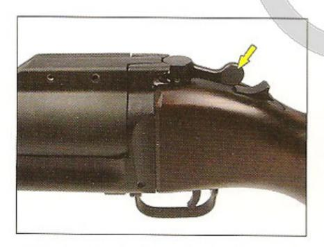
Closing the breech will cause the barrel locking latch to return to center.
