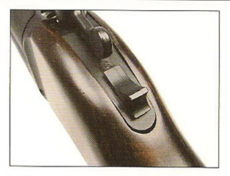
Safe: Pull the safety backward and the symbol "S" can be seen. The trigger cannot be pull at this position.
