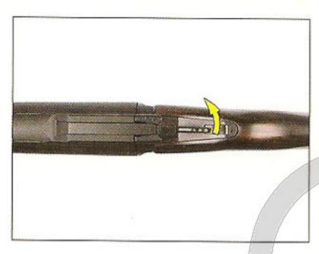
To load the launcher, push the barrel locking latch to the right and open the breech. Gravity will pull down the barrel, breaking it open, and exposing the breech.
