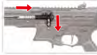
Be sure to have the rod facing down and reaching to the end. Remove clogged pellets.
