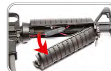
Remove the lower handguard.
