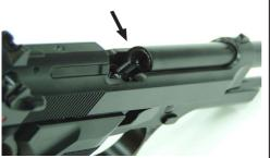
AFTER THE LAST SHOT IS FIRED, SLIDE WILL STOP IN THE REAR. CHECK THE CHAMBER AND MAKE SURE THE CHAMBER IS EMPTY.PRESS THE SLIDE STOP DOWN OUT OF ITS LOCKING NOTCH TO ALLOW THE SLIDE TO MOVE FORWARD.IF A LOADED MAGAZINE IS INSERTED AND THE SLIDE STOP IS PUSHED DOWN,THE SLIDE WILL LOAD A FRESH CARTRIDGE FROM THE MAGAZINE INTO THE CHAMBER, AND THE PISTOL IS READY TO FIRE.
