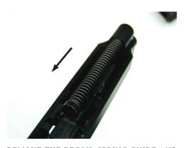
REMOVE THE RECOIL SPRING GUIDE AND SPRING.
